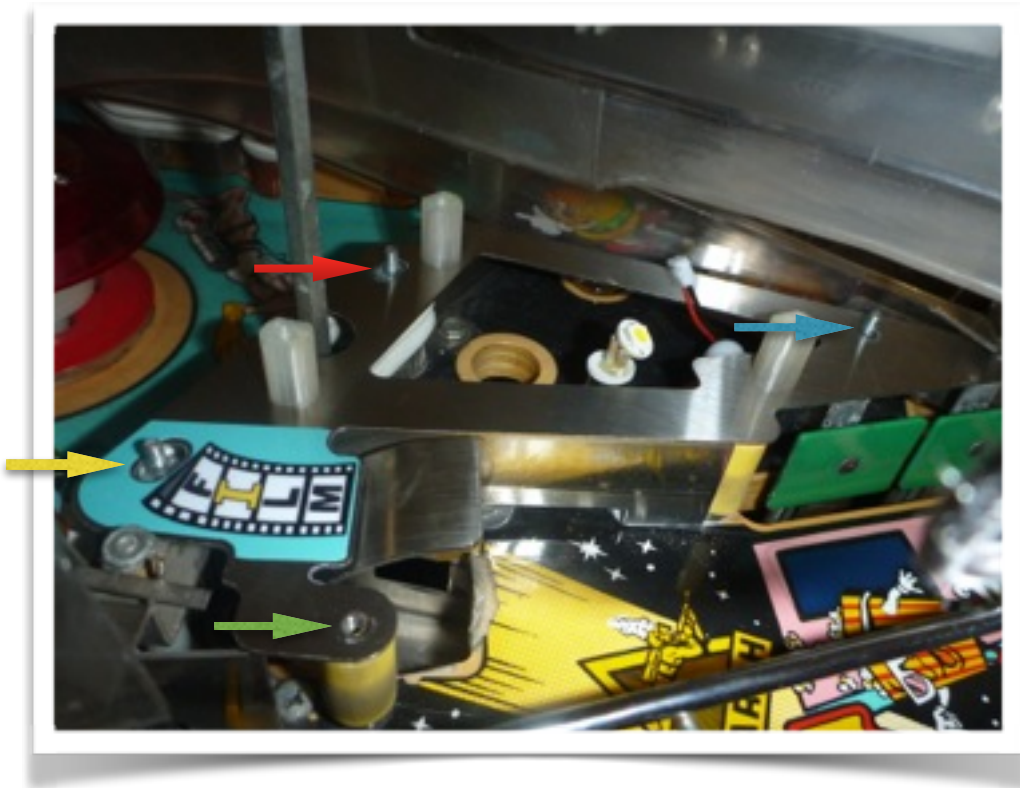
photo 9 - install the snackbar SS base plate over the 3 available screws.
