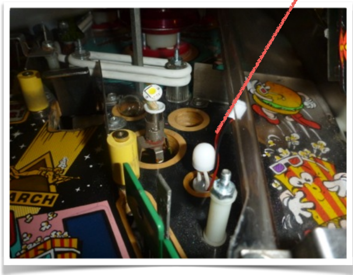
photo 8 - install the replacement GI globe which has a double adaptor lead also coming out of it.
