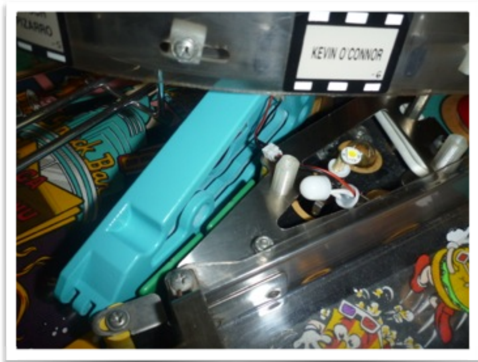
photo 13 & 14 - line up and pass through the GI bulb through the GI hole.
